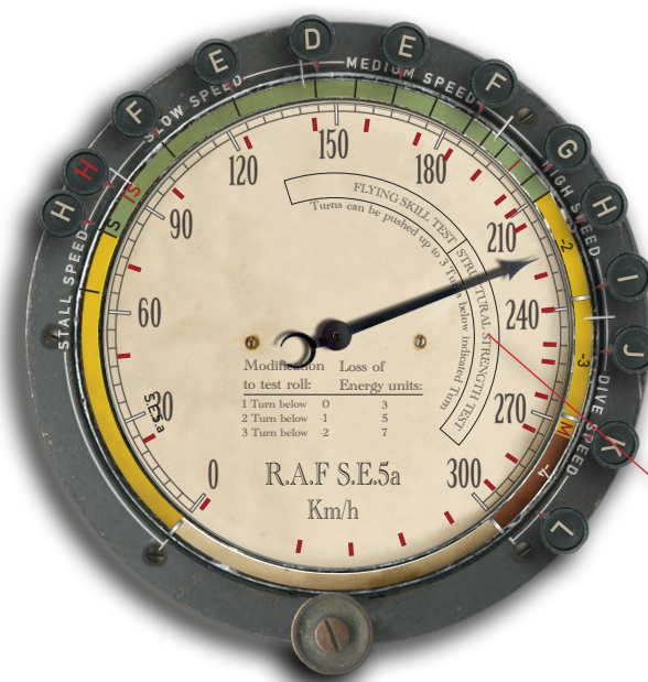
Illustration. The Modification Table found on the Cockpit panel of the S.E.5a
